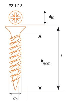
**The FFX Twin Threaded CSK Woodscrew.** Case hardened woodscrew with pozi drive recess head. It's Twin Thread enables faster installation with greater pull out loadings. The Sharp point ensures fast and accurate drilling.
